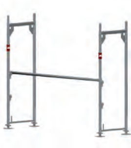
Assemble vertical frame and secure with guard rail
