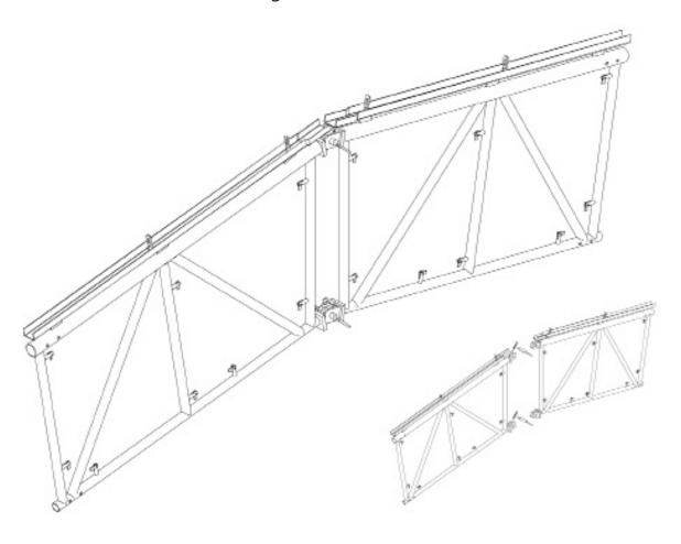
The structural stiffness of main and make-up trusses is realized by transverse frames secured to the parallel modular beams. SL Diagonals and guard rails to the lower chord are required according to the length of the trusses. For all connections of transverse frames, diagonals and guard rails the modular beams are equipped with gravity pins.
