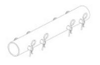
The modular beams are available in lengths of 1.0 and 2.0 m and are connected using tubular connection spigots secured with locating bolts and split pins.
